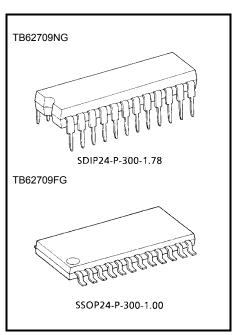
Weight SDIP24-P-300-1.78 :1.62 g (typ.) SSOP24-P-300-1.00:0.32 g (typ.)
